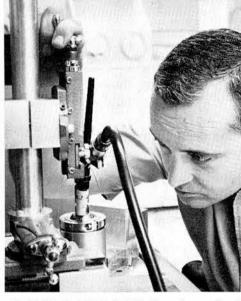
GEORGE EDGERLY (4221-2) performs final TIG (tungsten inert gas) welding on the assembled switch. Physical Electronics Lab performed tooling and fixture development for the switch in three months' time.
